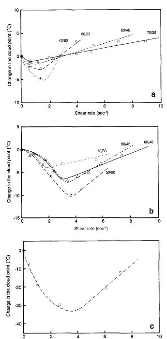
Figure 6 Change in the cloud point as a function of shear rate for (a) EVA/SCPE11 blend, (b) PBA/SCPE12 blend and (c) PS/PVME blend. Compositions are as shown in the figure
