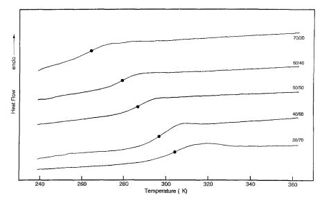
Figure 2 D.s.c. thermograms for the five indicated compositions of the PBA/SCPE12 blend. The glass transition temperatures are indicated by small black circles on the observed transitions
