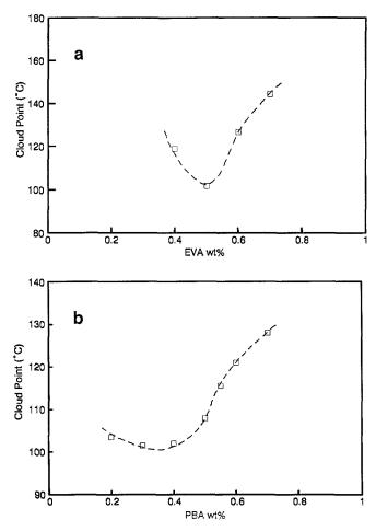
Figure 4 Cloud-point curves for (a) EVA/SCPE11 blend and (b) PBA/SCPE12 blend
