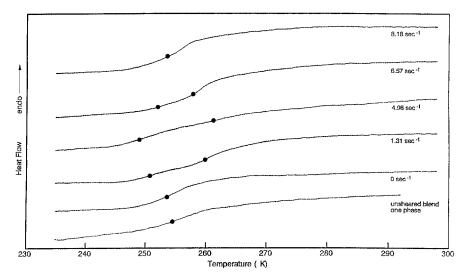
Figure 8 D.s.c. thermograms for five samples taken from different radial locations of a PS/PVME (30/70) blend sheared at  $\dot{\gamma}_R = 8.8 \, \mathrm{s}^{-1}$ . The glass transition temperatures are indicated by small black circles on the observed transitions
