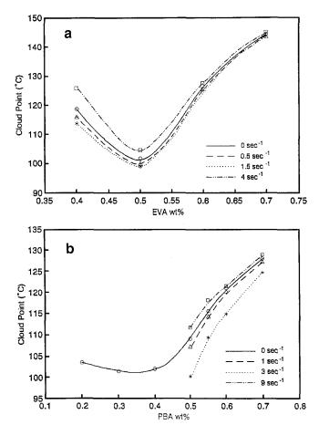
Figure 7 Dependence of the cloud-point curve on the applied shear rate for (a) EVA/SCPE11 blend and (b) PBA/SCPE12 blend. Data at  $9 \, {\rm s}^{-1}$  in (b) were obtained by extrapolation
