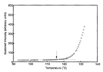
Figure 3 Determining the quiescent cloud point of a (55/45) PBA/SCPE12 blend using the light scattering data. The cloud point is indicated by the arrow
