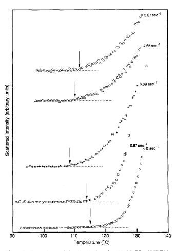
Figure 5 Dependence of the cloud point of a (55/45) PBA/SCPE12 blend on the applied shear rate. The cloud point is indicated by an arrow on each curve
